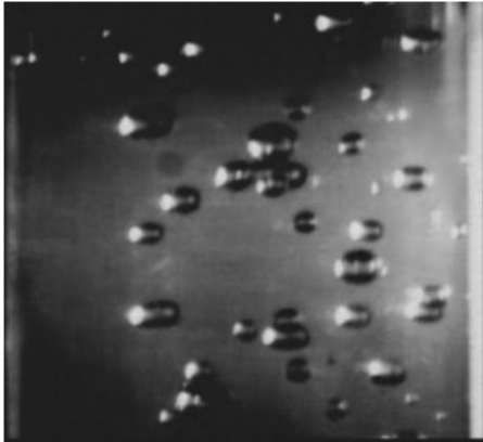
Figure 3: Discrete bubbles sub-regime ( \alpha = 1\% ).
