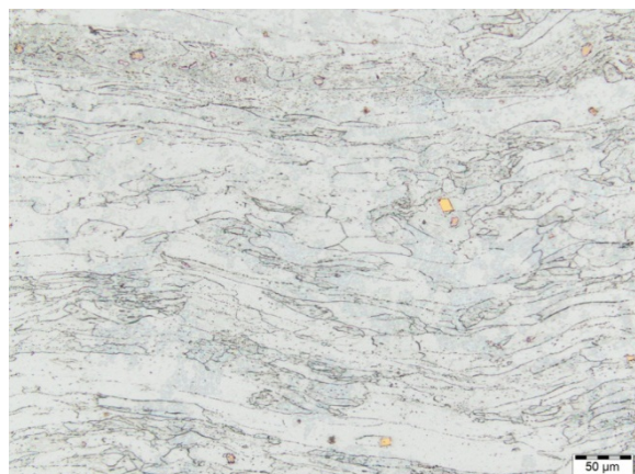
Figure 6-10: Optical micrograph of as-received hot band after etching with H 2 O, HCl and HNO 3 for 60 seconds
