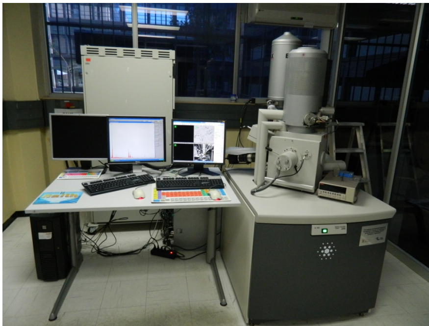
Figure 5-1: FEI NOVA NanoSEM 230 FEG used for analysis
