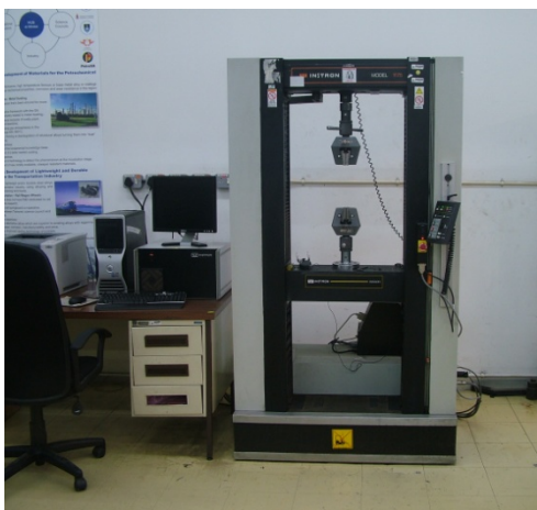
Figure 5-2: Instron tensile testing machine used to determine R_m -values and mechanical properties.
