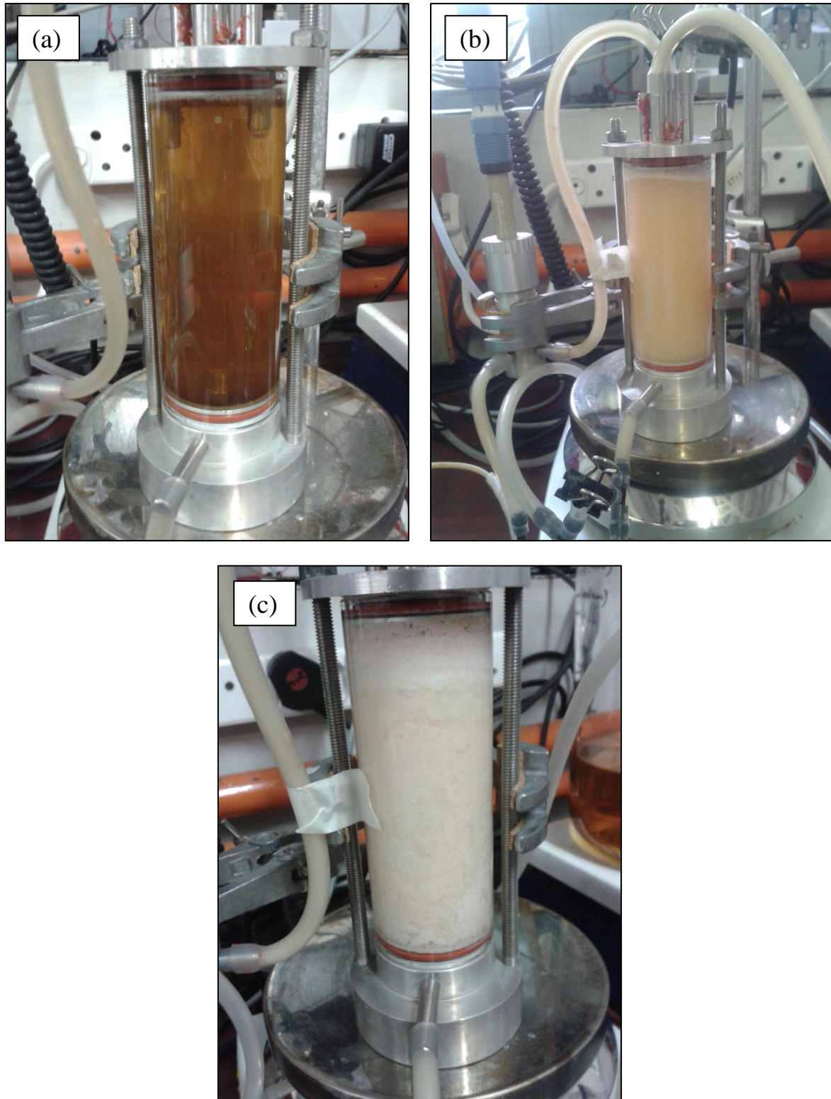
Figure 3.7: Images of Reactor A during various stages of fermentation: (a) before inoculation, (b) during growth but without biofilm formation, and (c) established biofilm on the reactor body (no packing)
