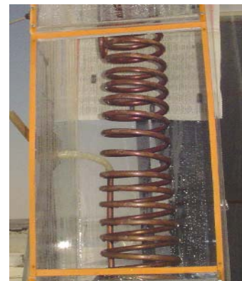
Fig 3. Condenser of setup (conical coil)[1]
