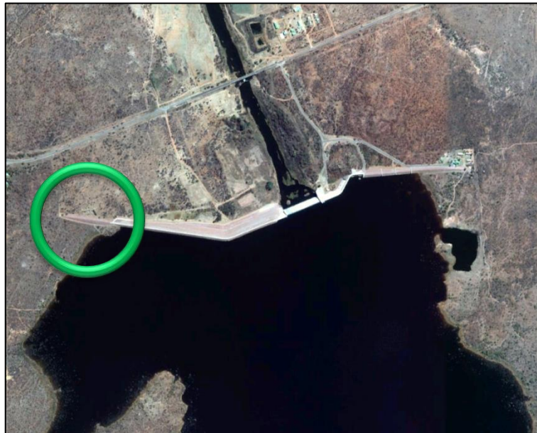
Figure 2-5: Arabie Dam, now called Flag Boshielo Dam in the Crocodile River, South Africa with limited service spillway embankment to be flushed away under large floods without damaging the main spillway structure
