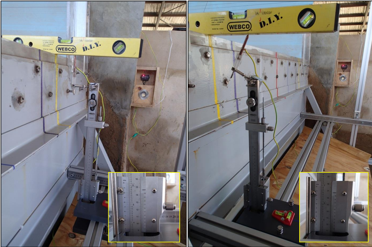
Figure 3-30: Vertical displacement of the copper tip of the OPMI relative to the crest of the weir (vertical - left, rotated - right)
