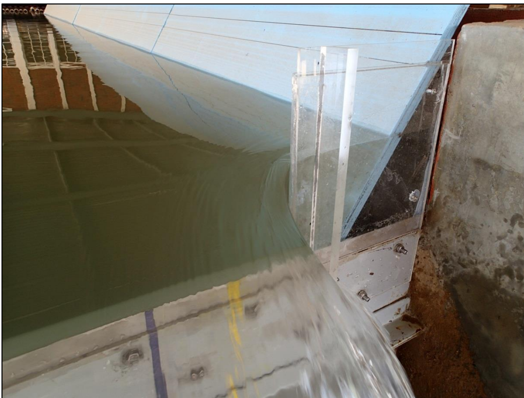
Figure 4-14: High flow velocities experienced at boundary of sharp-crested weir's crest caused by the steep inclination of the 60° side wall
