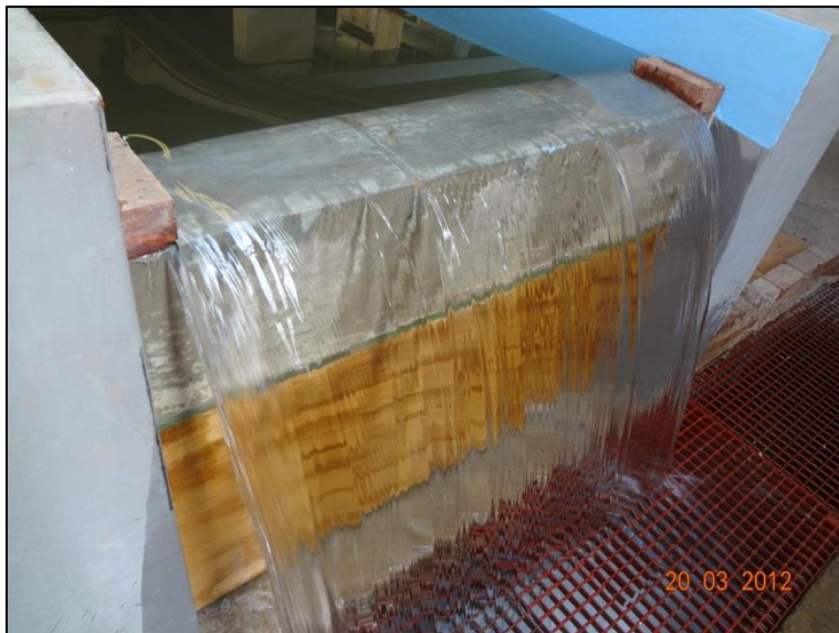
Figure 3-19: Existing physical model of free falling weir at the Department of Water Affairs Hydraulic Laboratory
