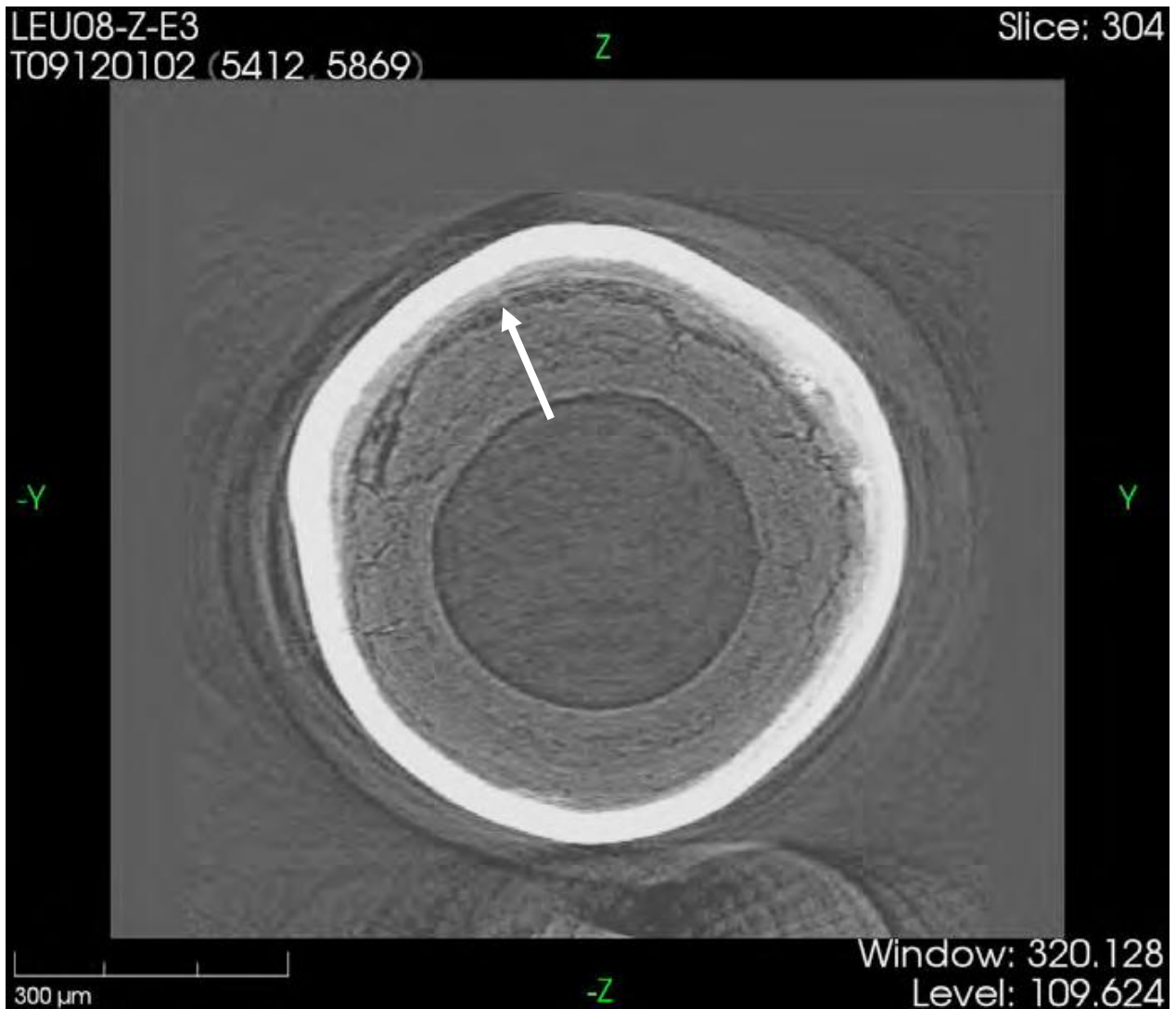
Figure 5.13a: High resolution x-ray tomography of a SiC defect particle after the kernel was removed by acid leaching at ORNL. The white ring shows the SiC layer, the damaged porous layer below the white ring pointed by the arrow is the IPyC layer.
