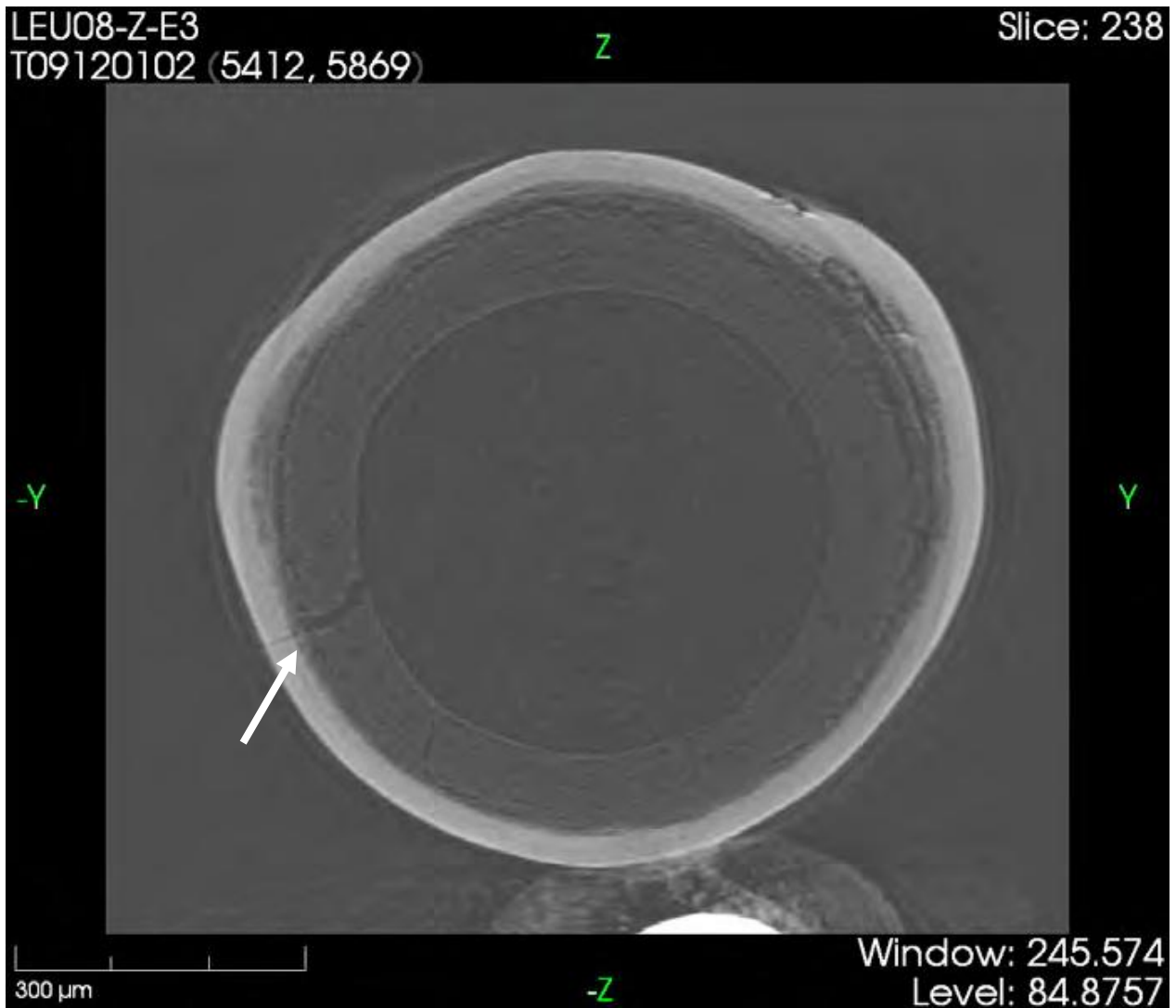
Figure 5.13b: The same particle as in Figure 5.13a showing a crack in the SiC layer (arrow).
