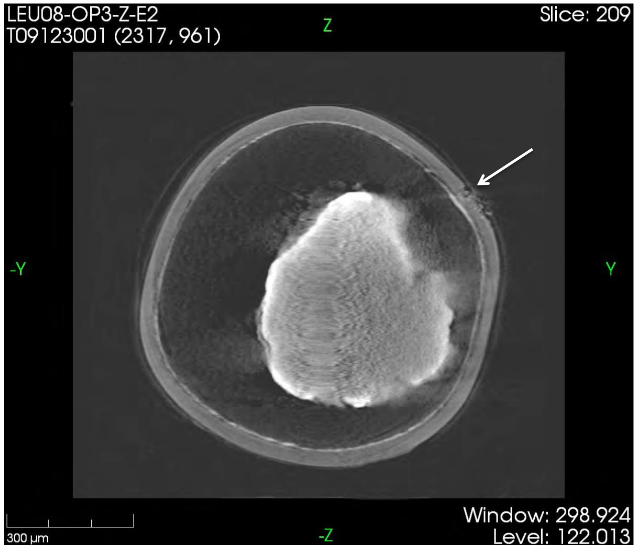
Figure 5.14: High resolution tomography of a SiC defect after the kernel was partially removed by acid leaching.
