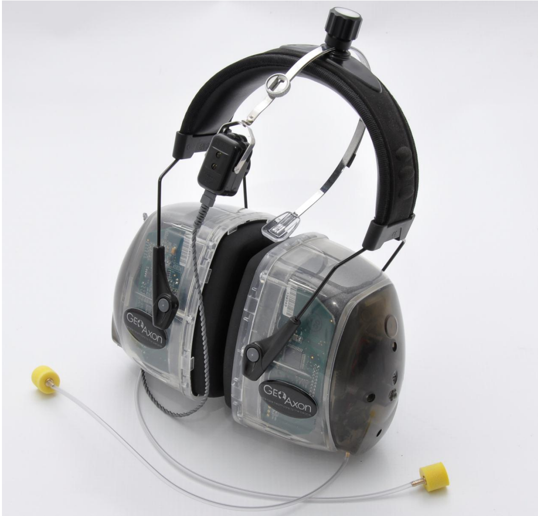
Figure 2.1 KUDUwave audiometer showing insert earphones, circumaural earcups housing audiometers and forehead bone conductor mounted centrally on headband
