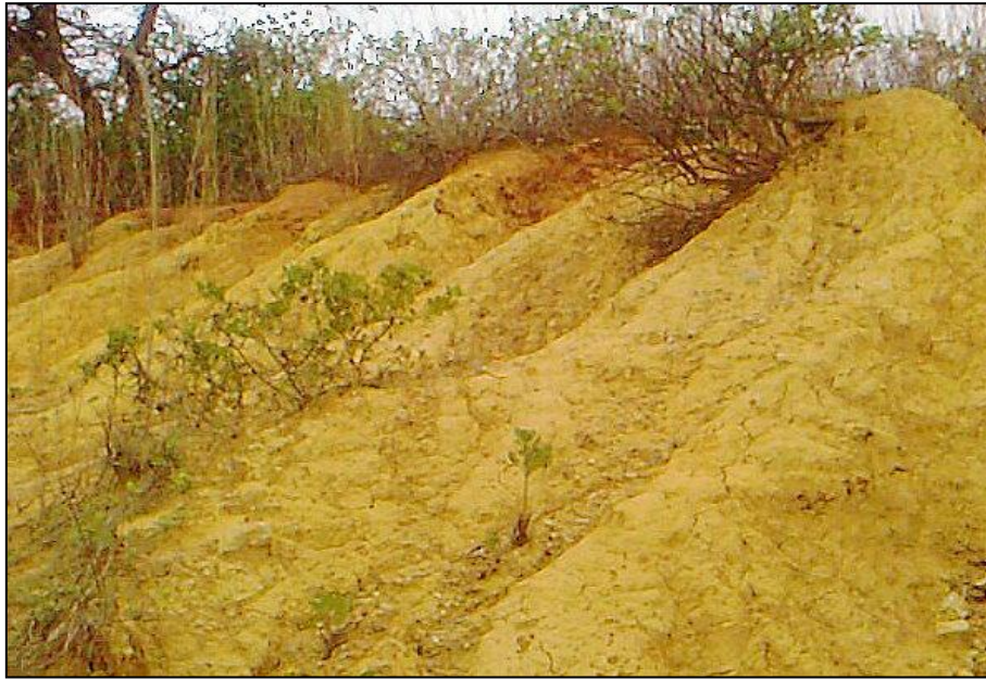
Figure 3-2: Suspected moderately dispersive sample (COED1) with erosional channels.
