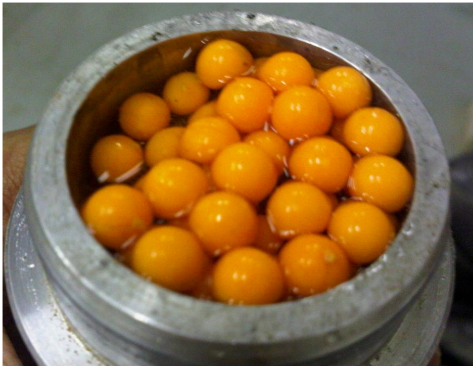
Figure 6-3: Photograph showing the accumulation of water in the pea gravel on top of the compacted specimen.
