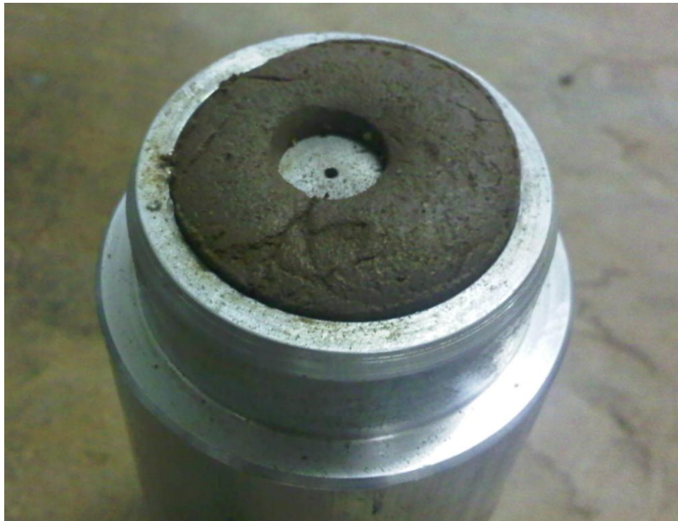
Figure 6-2: Photograph demonstrating the collapse of the nipple into the specimen.
