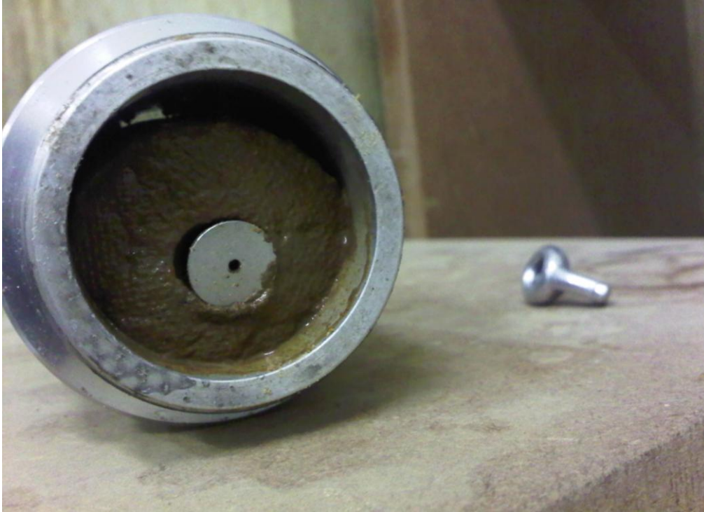
Figure 6-1: Photograph illustrating the collapse of sample UM108 into the cylinder.
