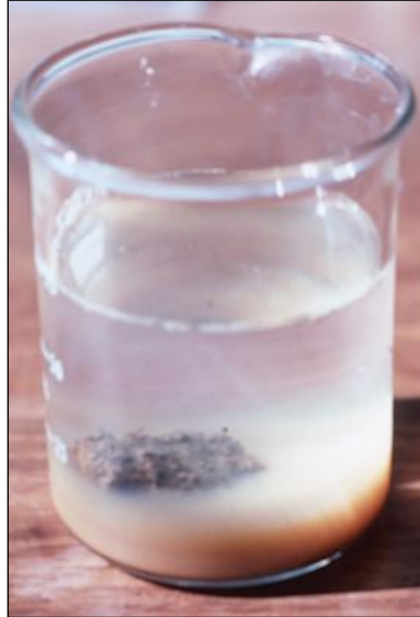
Figure 4-2: Colloidal suspension of a highly dispersive soil- Grade: 4- strong reaction (Courtesy of Paige-Green, 2010).
