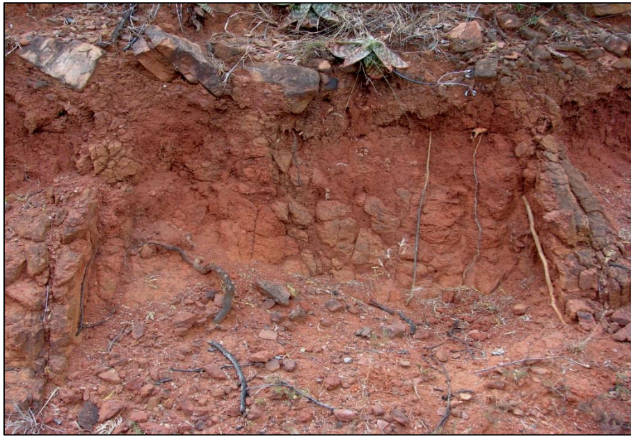
Figure 3-1: Non-dispersive sample (ND309) with no evidence of erosion, piping or gullies.
