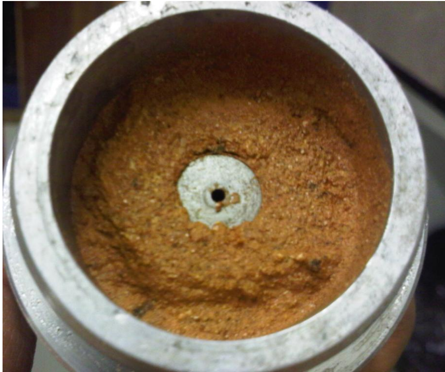
Figure 6-4: Photograph showing erosion of sample at the top end of the compacted specimen.
