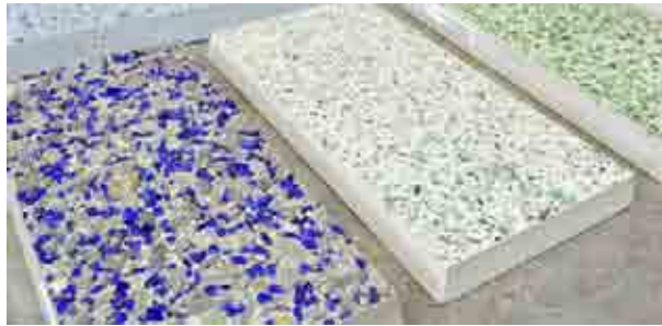
Illustration 184: Exposed glass aggregate concrete (BetonBild, n.d.).
