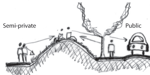
Illustration 144: Berms are a social way of defining a edge but also creating a visual screen (Author, 2012 from van der Walt, 2009).
