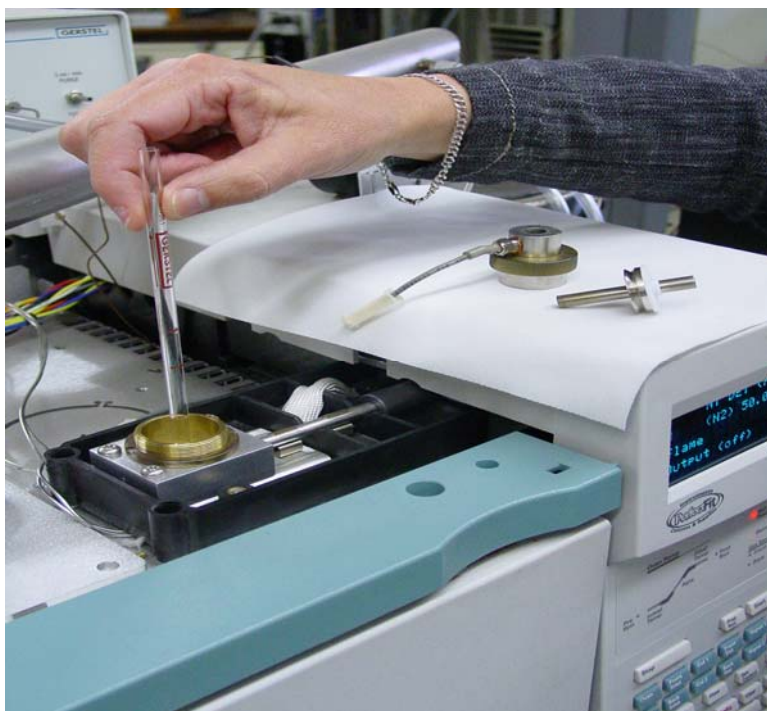
Figure 5.2. Removed detector top assembly and collector. MCT placed on GC-FID flame tip to recapture single peaks or various fractions [25]. Helium was used as the make-up gas.
