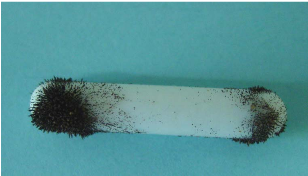
Figure 4.7b. Magnetic stir bar with magnetic soil particles accumulated from 40 g soil collected between the circles (Matrix 1.3). See section 4.3.4 for details.
