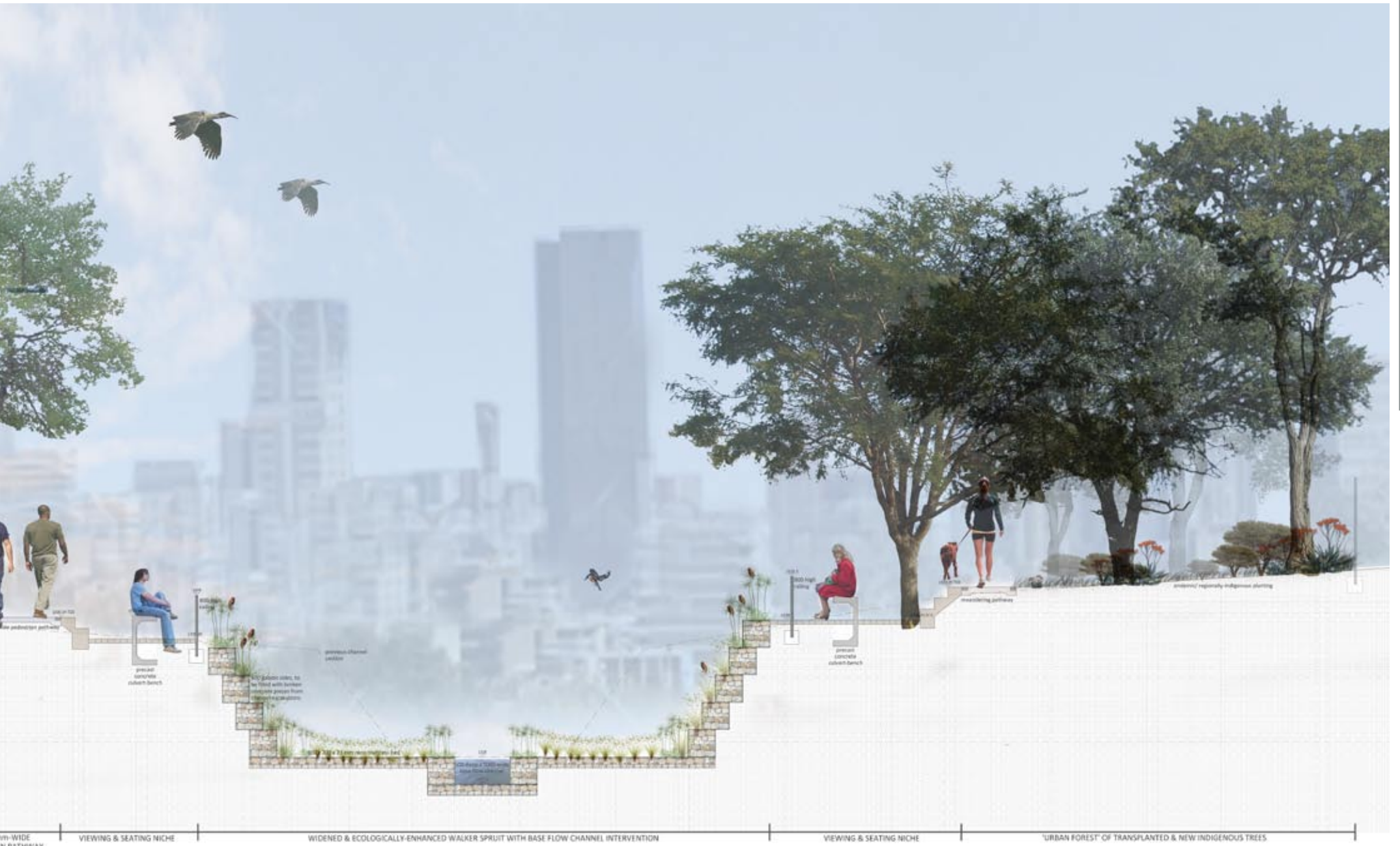
wide pedestrian path-way | viewing & seating niche | widened & ecologically-enhanced walker spruit with base flow channel intervention | viewing & seating niche | urban forest of transplanted & new indigenous trees
