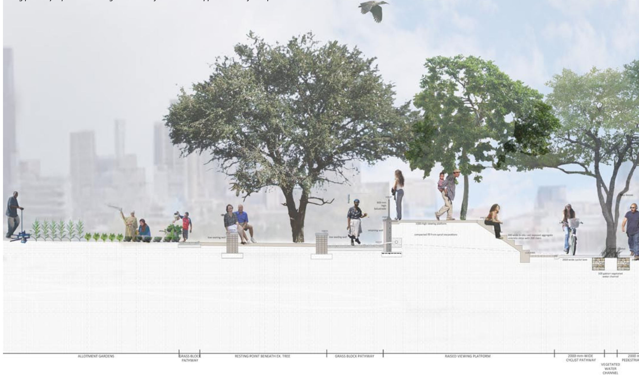
Illustration 279: Section F-F indicating one of the raised platforms, the pedestrian and cyclist pathways, and the de-channelized Walker Spruit alongside the urban forest (Author, 2012).
