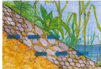
Illustration 34: Reno Mattress intervention (Maccaferri Gabions, 2001:3)
