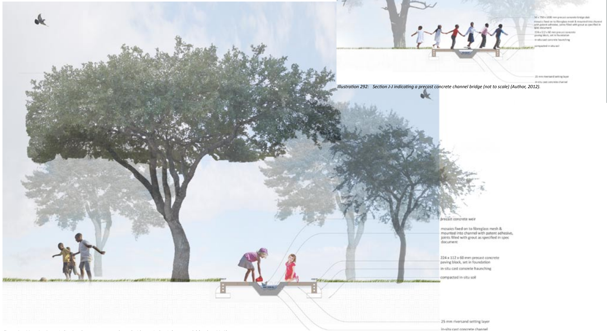
Illustration 291: Section I-I indicating the open concrete channel with a typical weir (not to scale) (Author, 2012).
