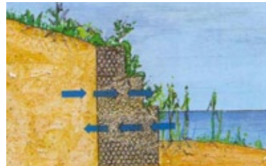
Illustration 35: Stacked gabion intervention (Maccaferri Gabions, 2001:3)
