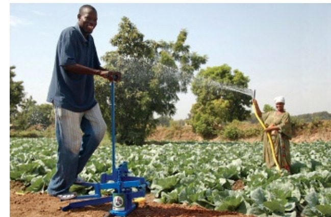
Illustration 198: Providing the pressure needed for a hose via the use of a low-tech treadle pump (From: https://www.engineeringforchange.org/news/2012/01/23/ten_low_tech_ways_to_irrigate_crops.html )
