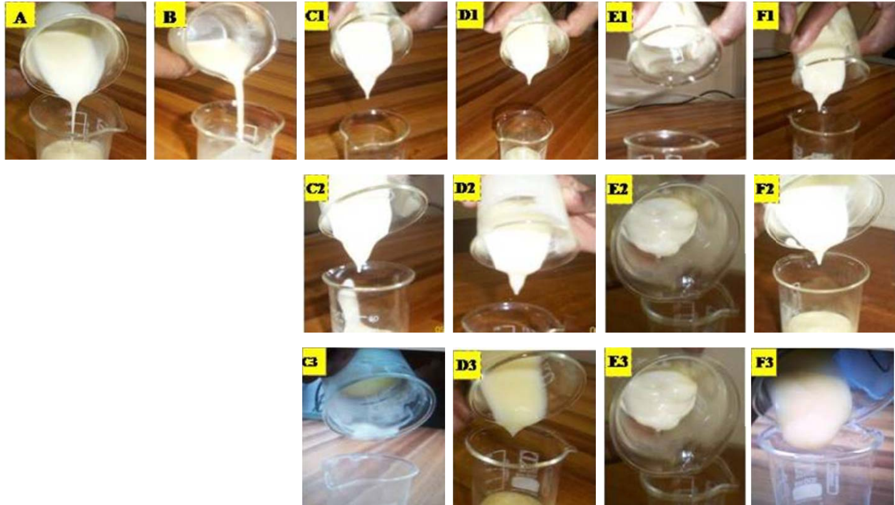
Figure 4.2: Pictures showing pouring ability from a beaker of each mayonnaise sample 30 minutes after their preparation. A-full fat mayonnaise, B-50% oil reduced product with no starch added, C1,C2,C3- LCMTEs with unmodified teff starch at 50%, 80%, and 100% oil replacement respectively, D1,D2,D3- LCMTEs with teff starch modified with 1.5% stearic acid at 50%, 80%, and 100% oil replacement respectively, E1,E2,E3- LCMTEs with unmodified maize starch at 50%, 80%, and 100% oil replacement respectively, F1,F2,F3- LCMTEs with maize starch modified with 1.5% stearic acid at 50%, 80%, and 100% oil replacement respectively
