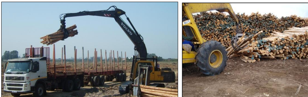
Figure 12: Knuckle-boom loader, and Figure 13: Three-wheeled loader
