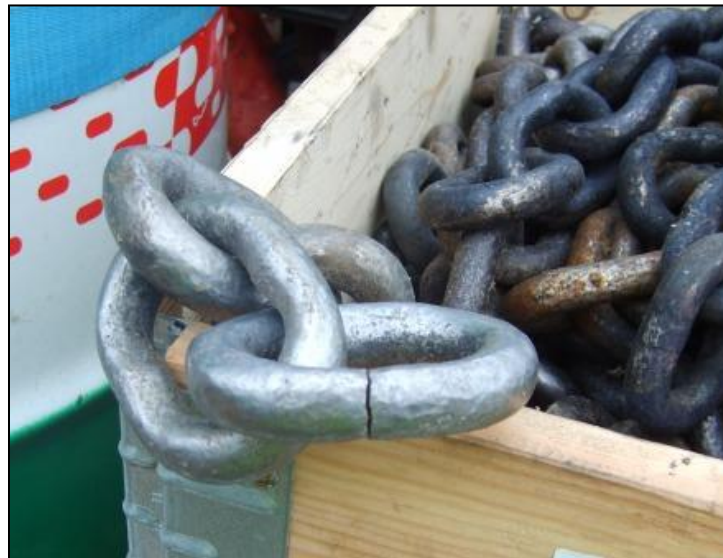
Figure 15: Chain link failure at the weld
