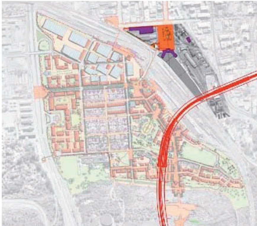
Figure showing alignment of the proposed Gautrain system tunnelled through Salvokop and the Pretoria Station Precinct
