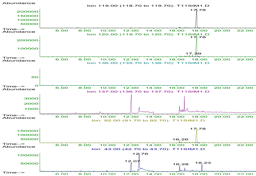
Figure 4.2: The Extracted Ion Chromatogram of the Diethyl Ether Extract of one of the five Tablets extracted in Test Case 1, run on the SIM 1 method. The following masses were extracted: 119, 120, 136, 137, 92 and 43.
