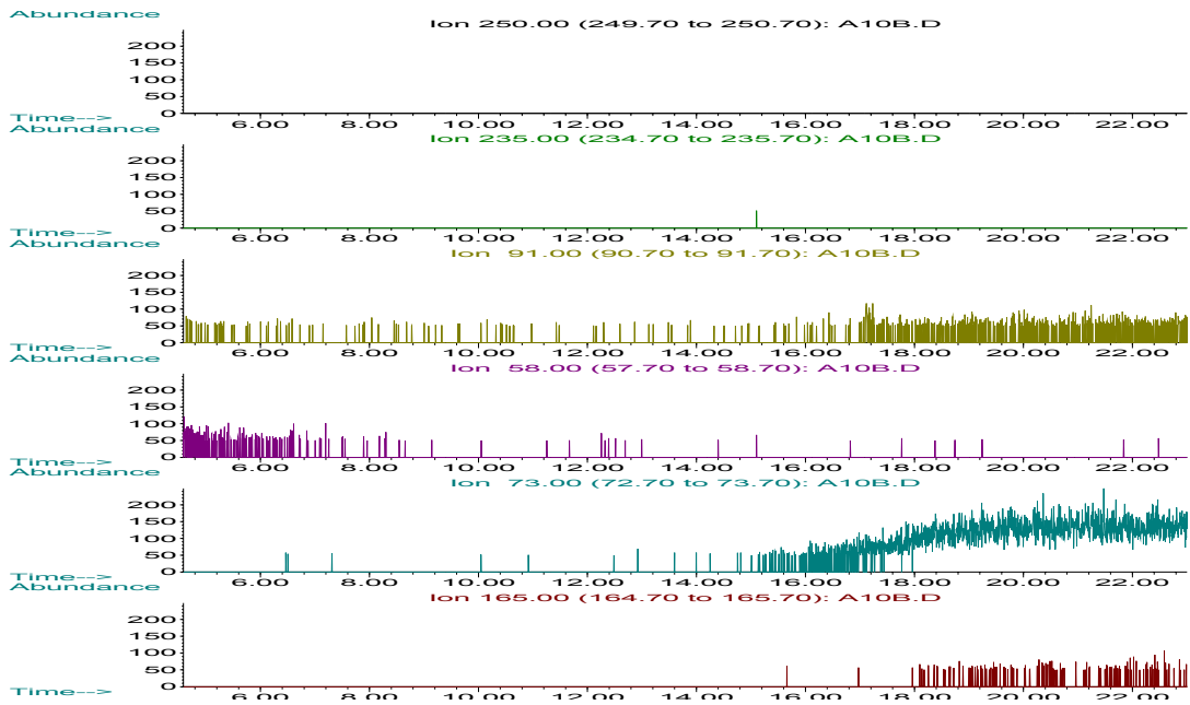
Figure 3.47: An example of the extracted ion chromatogram for Methaqualone (ions 235 and 91) and Diphenhydramine (ions 58, 73 and 165) of the chloroform blank for the 10 th tablet in Test Case 2. No methaqualone or diphenhydramine contamination is present.
