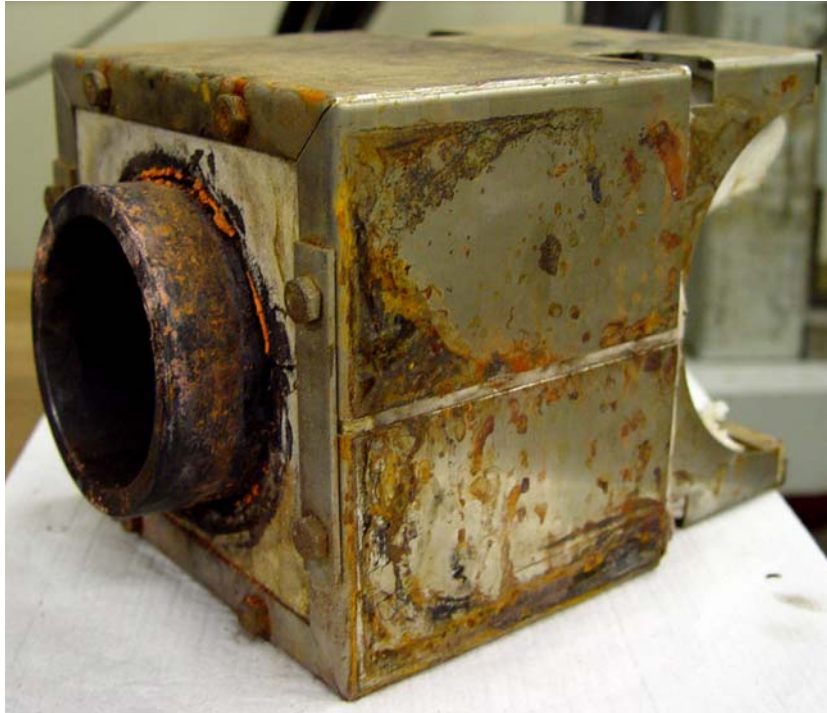
Figure 5.12. The environmental chamber to heat the cantilever beam
