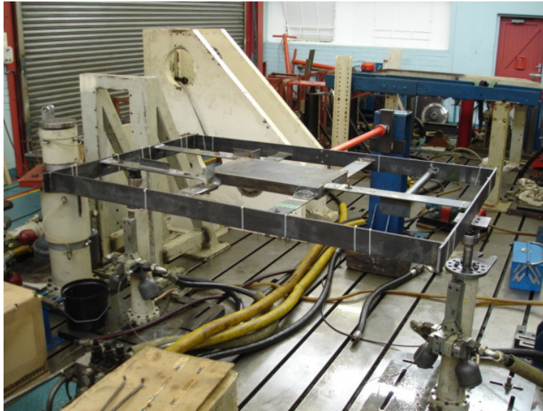
Figure 3.12: H-frame mounted on the test block with actuators, constraints and strain gauges.
