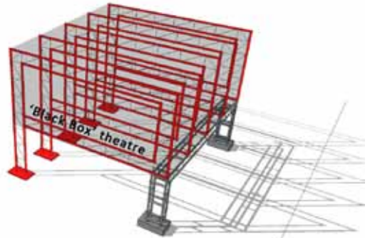
Figure 198 - diagram of primary trusses spanning the width of the building and supported by the steel beam structure on the one side.
