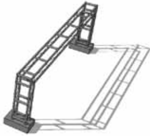
Figure 197 - diagram of the supporting steel beam structure used to support the primary trusses of the 'Black Box' theatre.
