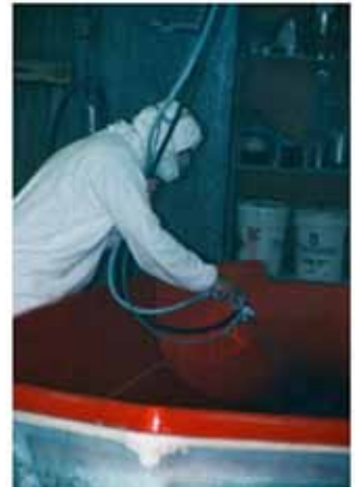
Figure 208 - image of gel coat being applied.
