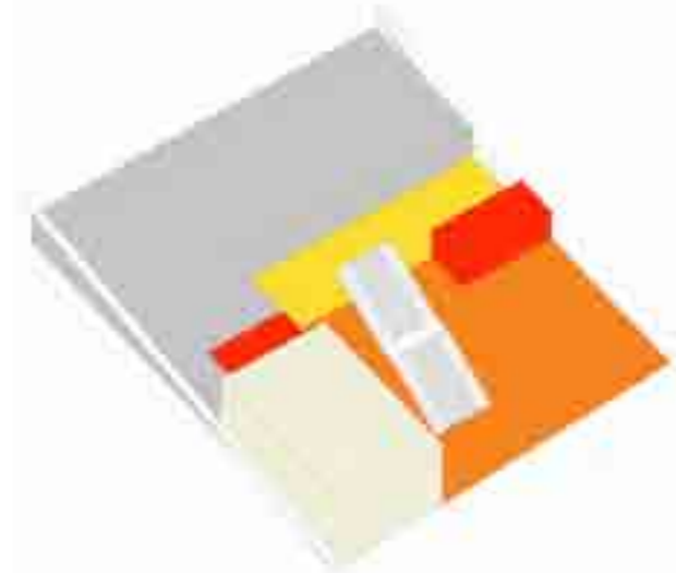
fig. 77_ Spatial diagram indicating relationship of main stair and atrium to other functions
