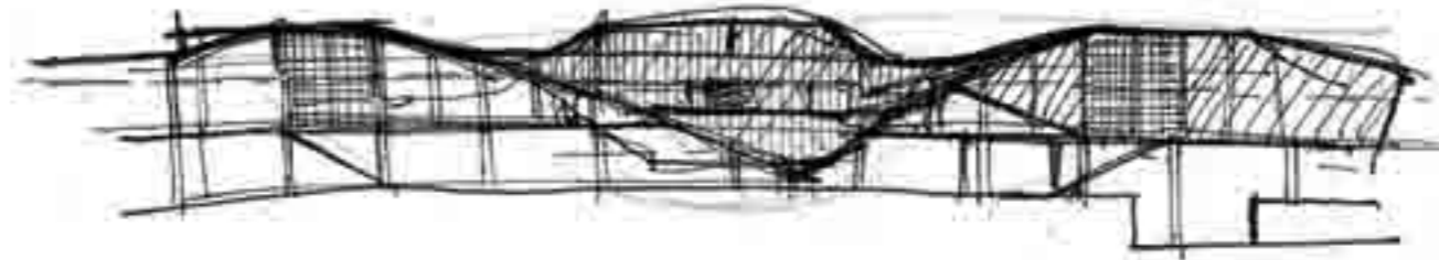
fig. 121_ Conceptual design development of platform roof and facade becoming more open to reveal the platform, allow for views and break the monotonous facade.
