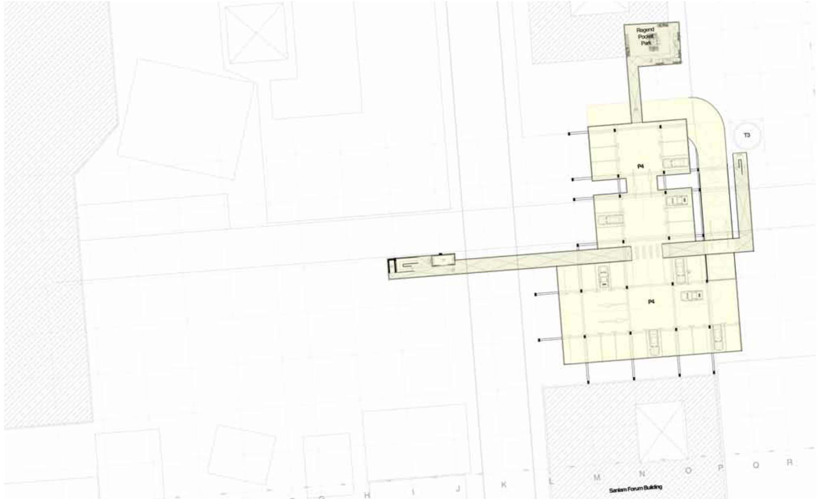
[Figure 8_12.] Seventh Floor Plan, showing the fourth parking floor with 30 parking bays. Regend Place pocket park and connection bridge.
