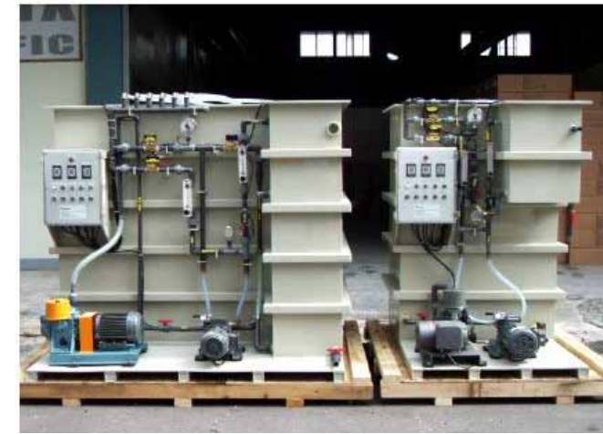
[Figure 4_2.] Wock Oliver model VOK MBR 2.5m X 2m X 2.2m, will be suitable for on site needs.
