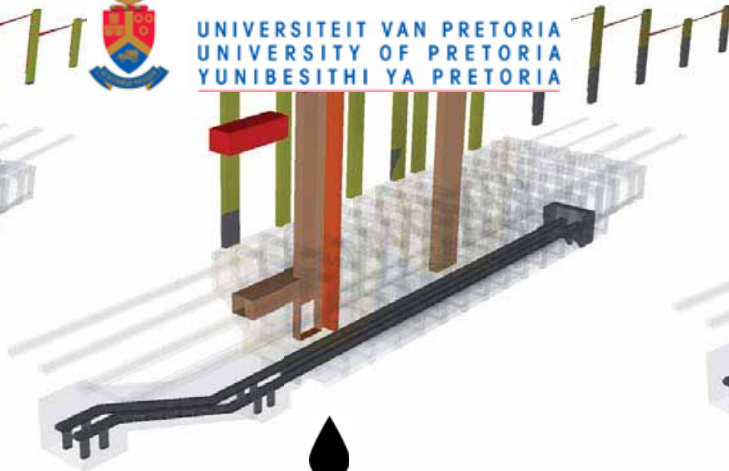
sewerage shafts; biogas reactor, UV radiation and micropore filter chambers
