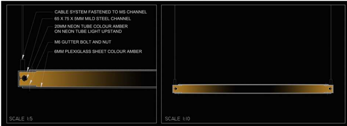
DETAIL SUSPENDED ILLUMINATED BULKHEAD (CIRCULATION LIGHTING ELEMENT)
