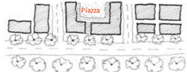
Fig 1.27 Proposed scenario with building in fill to create continuity
