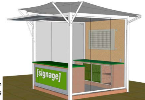
Rectangular steel structural frame with bolt-on corner posts for tensile fabric fixing
