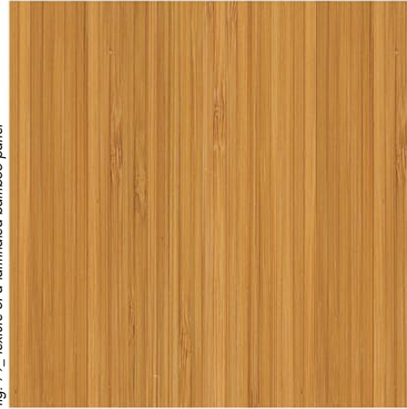
fig. 79_ texture of a laminated bamboo panel
