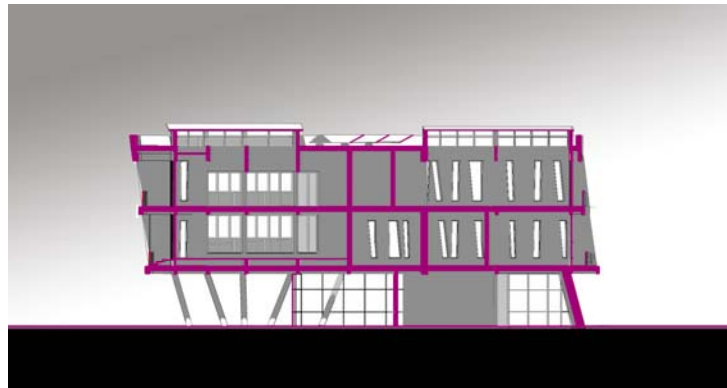
Figure 7-15: Summer noon solstice sunlight penetration on the Eastern Wing (Source: Own Image)
