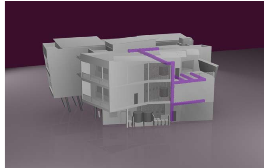
Figure 7-2: HVAC-System Ducting (Source: Own Image)
