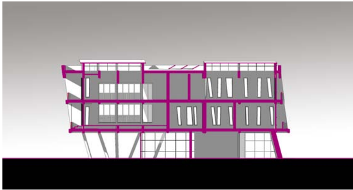
Figure 7-14: Winter noon solstice sunlight penetration on the Eastern Wing (Source: Own Image)
