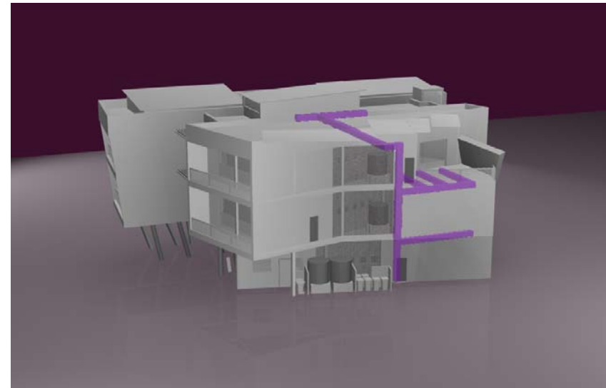
Figure 7-2: HVAC-System Ducting (Source: Own Image)
