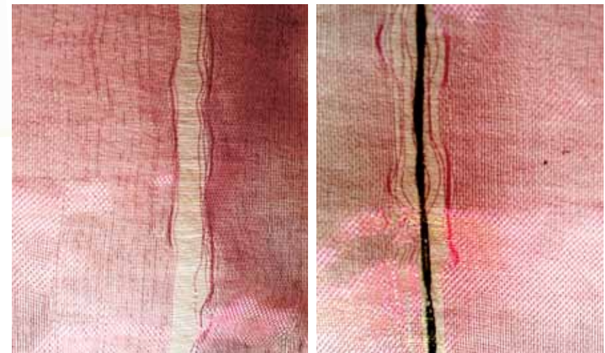
Figure 6.2: Photographs demonstrating how a yarn can be pulled out of a fabric and be replaced with a new yarn. (Author, 2012)
