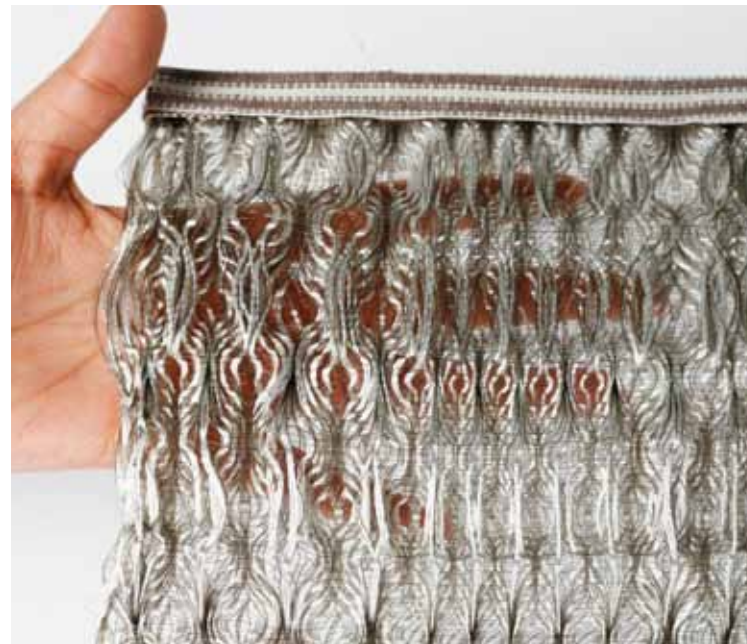
Figure 1.10: Honeycomb intersection from Textile Dimension. This fabric is 3D although it was woven on an ordinary 2D loom. (Garg, 2011)
