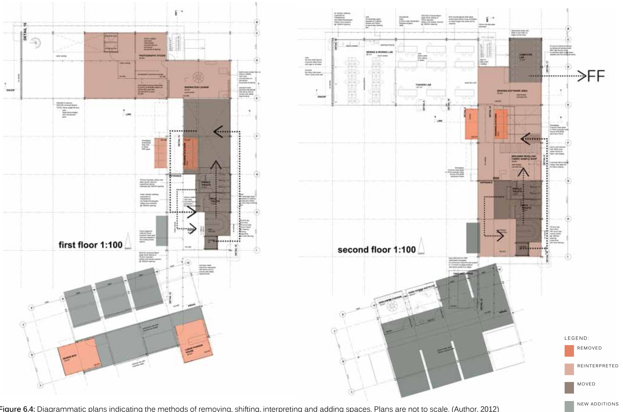
Figure 6.4: Diagrammatic plans indicating the methods of removing, shifting, interpreting and adding spaces. Plans are not to scale. (Author, 2012)
