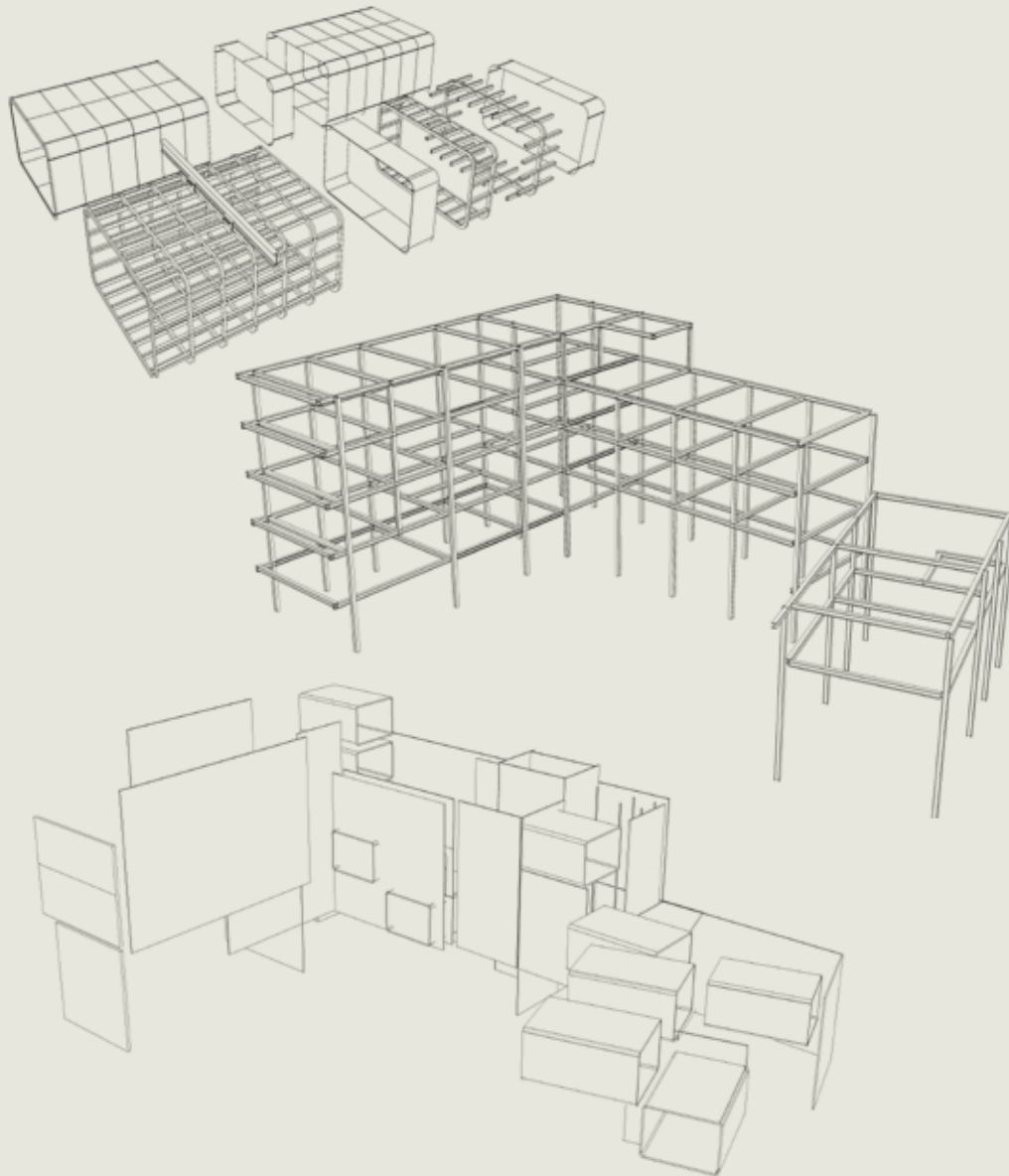
Figure 2.29: Diagrammatic models indicating the 'skin and bone' structure of the building (Author, 2012)
