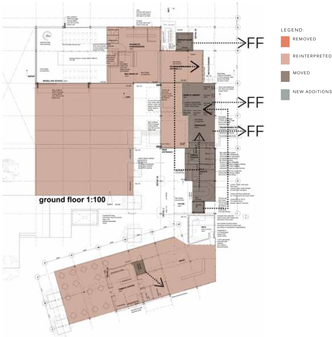
Figure 6.3: Diagrammatic plan indicating the methods of removing, shifting, interpreting and adding spaces. Plans are not to scale. (Author, 2012)
