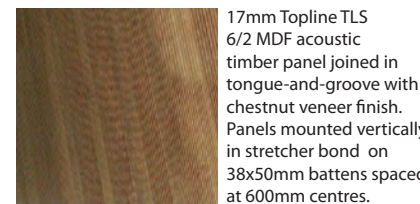
Fig.7.14 Acoustic timber veneer
