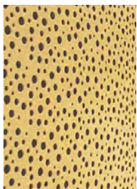
Fig.7.4 Acoustic panel with felt backing
