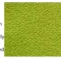
Fig.7.15 Acoustic fibreglass panel'
