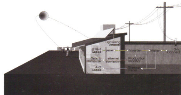
fig. 7.22 : Diagram of Dual Axis Photovoltaic Grid Intertie.
