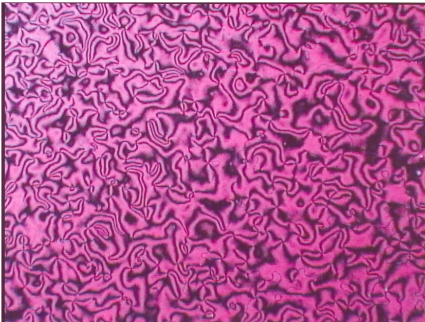
Figure 2.18 Nematic phase of [\text{Ni}(\text{S}_3\text{CTC}_8\text{H}_{17})(\text{S}_2\text{CTC}_8\text{H}_{17})] 3b at 105^\circ\text{C} (200 x magnification)
