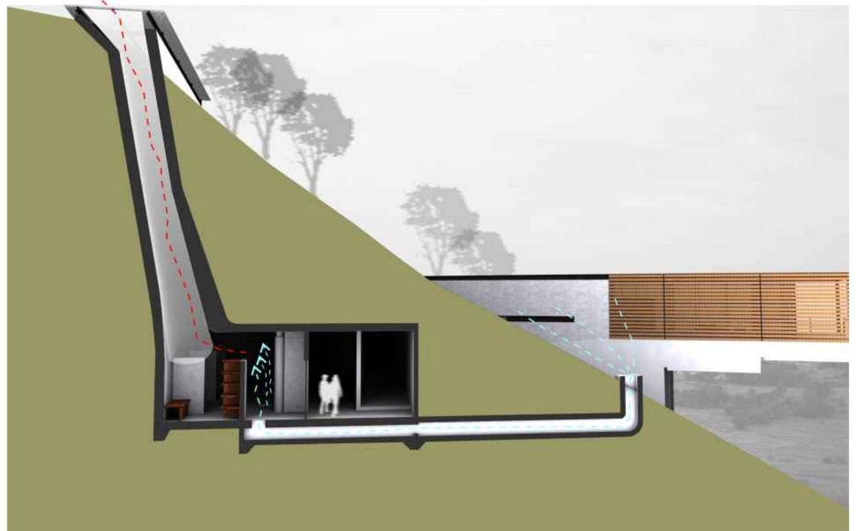
fig. 6.25. Passive ventilation through the Archaeological Research Centre. (2010)
