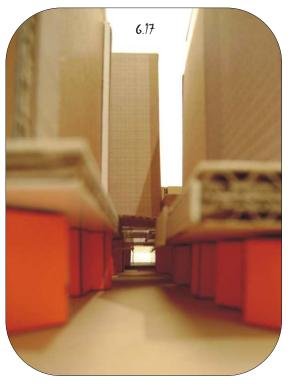
Areas for street vendors are designed as part of the edge and woven in between the retail spaces. The street vendor platforms will be raised from the arcade floor to provide space for lighting along the bottom edge, supplemented by an Illumesh backdrop. Vendor platforms that are unoccupied in the evening therefore create extra, well-lit lingering space for the night-time city dweller. The Illumesh backdrop provides advertising opportunity.
