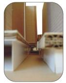
The redesign of the edge with alternating levels visually opens up the arcade. In perspective it seems much wider even though the building edge was not moved back.
