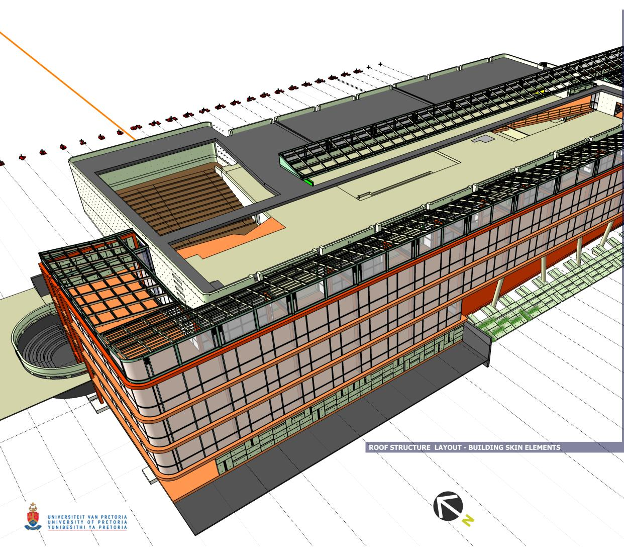
roof structural framework ex - 200x75 steel channel sections welded together in lattice format and fixed to existing concrete facade at shutter hole positions with ramset (or equal) chemical anchors
