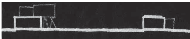
figure 8.4 diagrammatic section differentiating between stereotomic and tectonic structures
