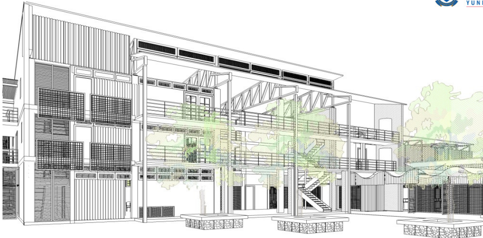
Figure 8.3 Circulation walkways connecting with exterior space with modular steel balustrades
