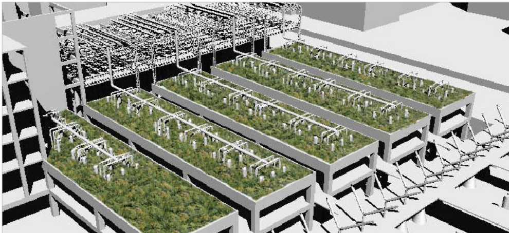
Fig 2.1.1.4: Skylights through green roof
