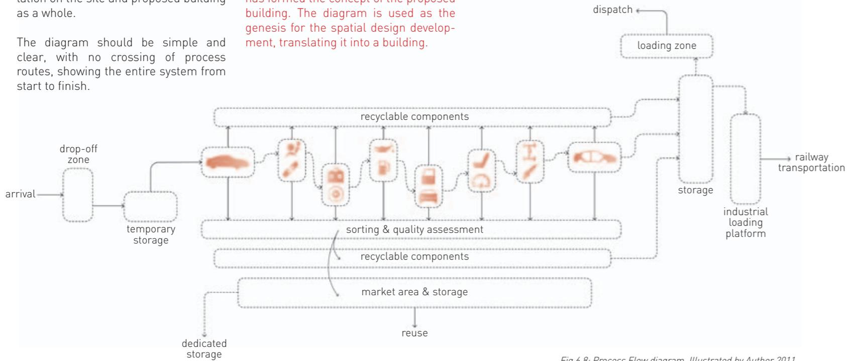
Fig 6.8: Process Flow diagram, Illustrated by Author 2011
