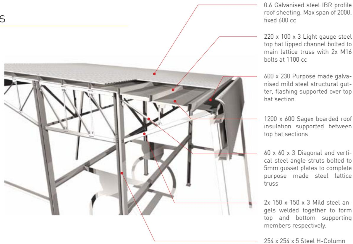
Fig 7.12: Perspective view of the primary structure's composition, Illustrated by Author 2011
