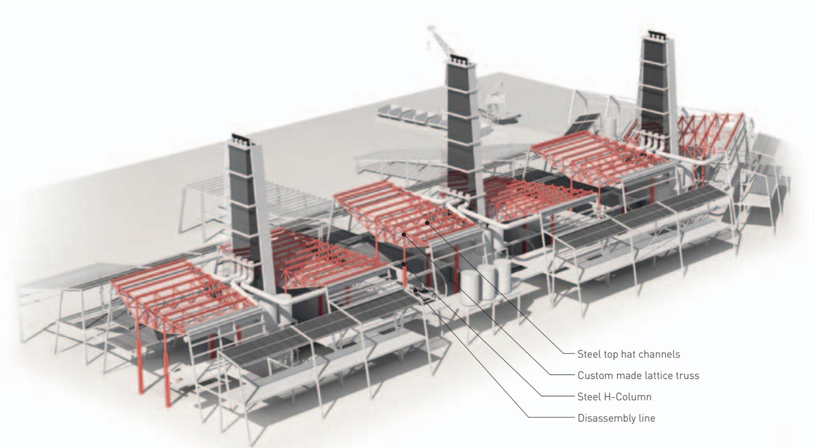
Fig 7.13: Position of the primary structure system within the proposed building, Illustrated by Author 2011
