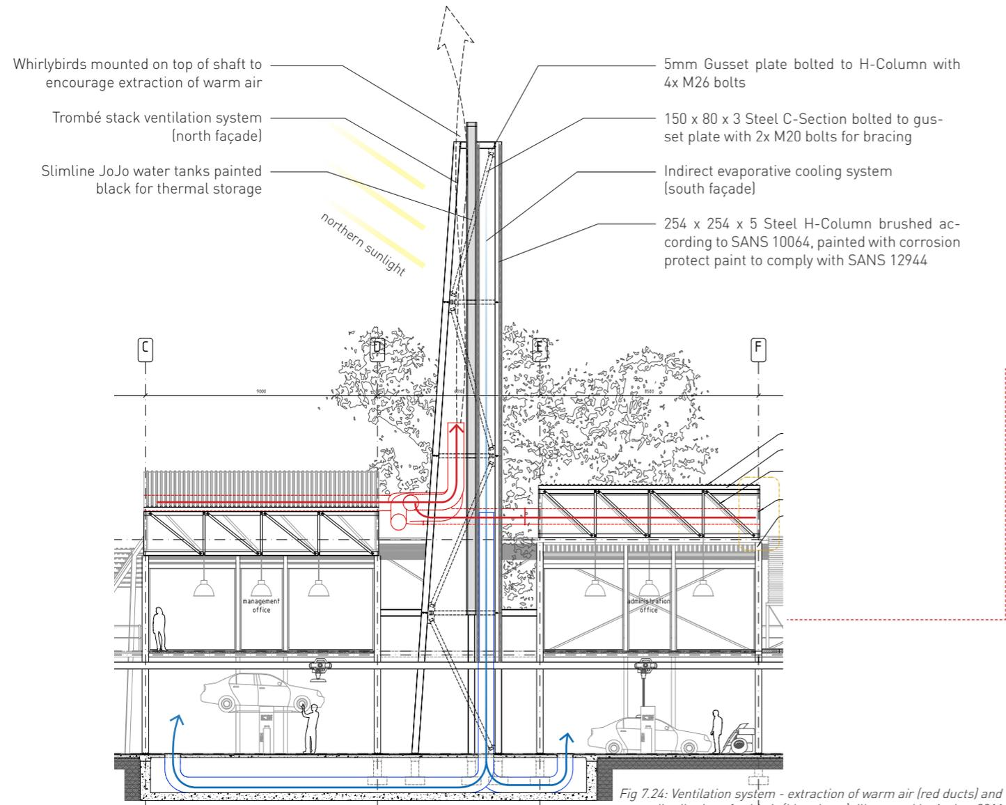
Fig 7.24: Ventilation system - extraction of warm air (red ducts) and distribution of cold air (blue ducts), Illustrated by Author 2011
