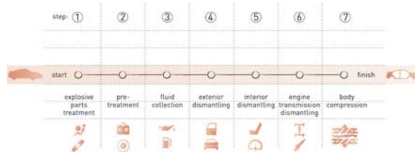
Fig 6.21: (Top) Disassembly line, Illustrated by Author 2011
