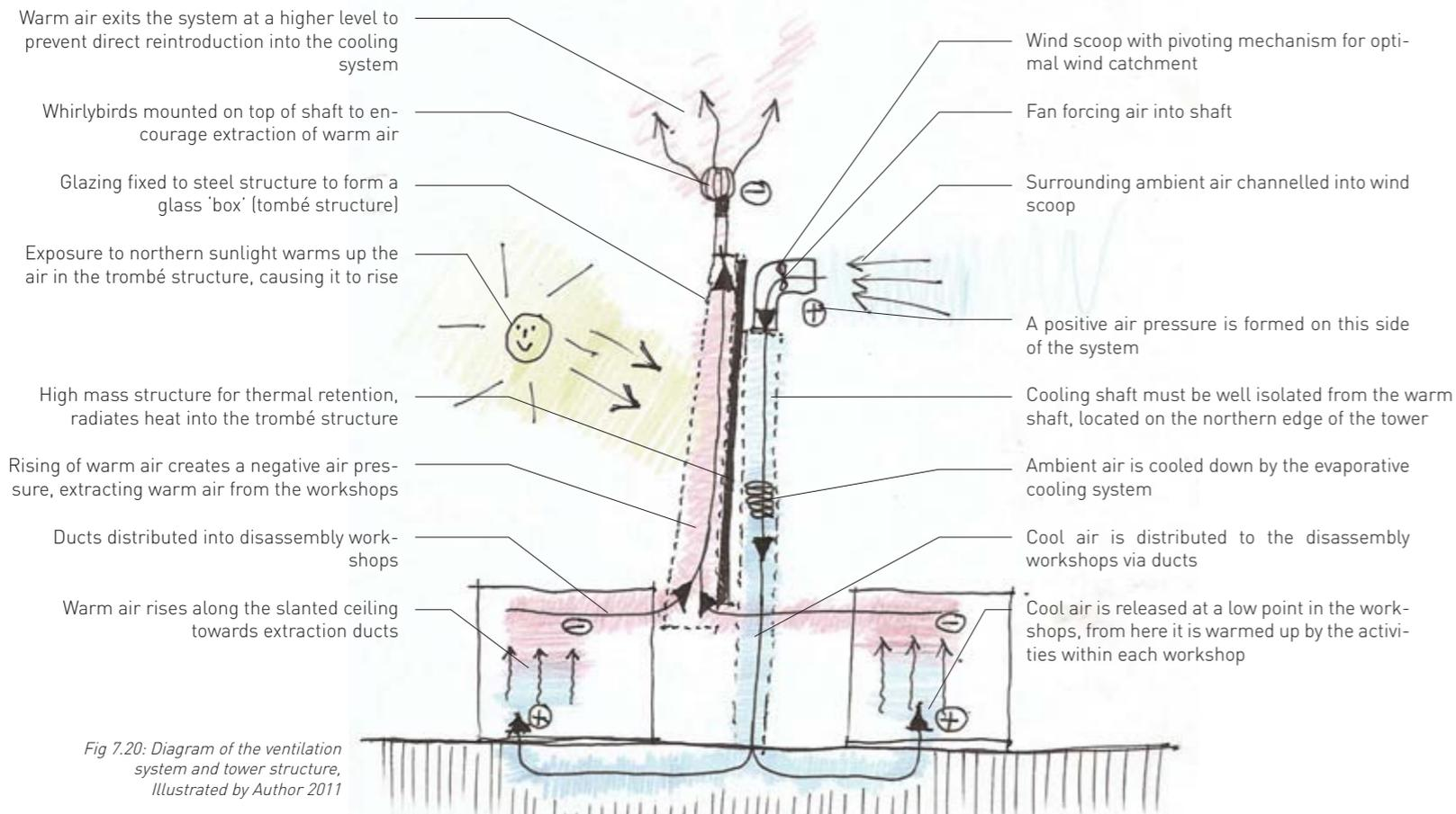
Fig 7.20: Diagram of the ventilation system and tower structure, Illustrated by Author 2011
