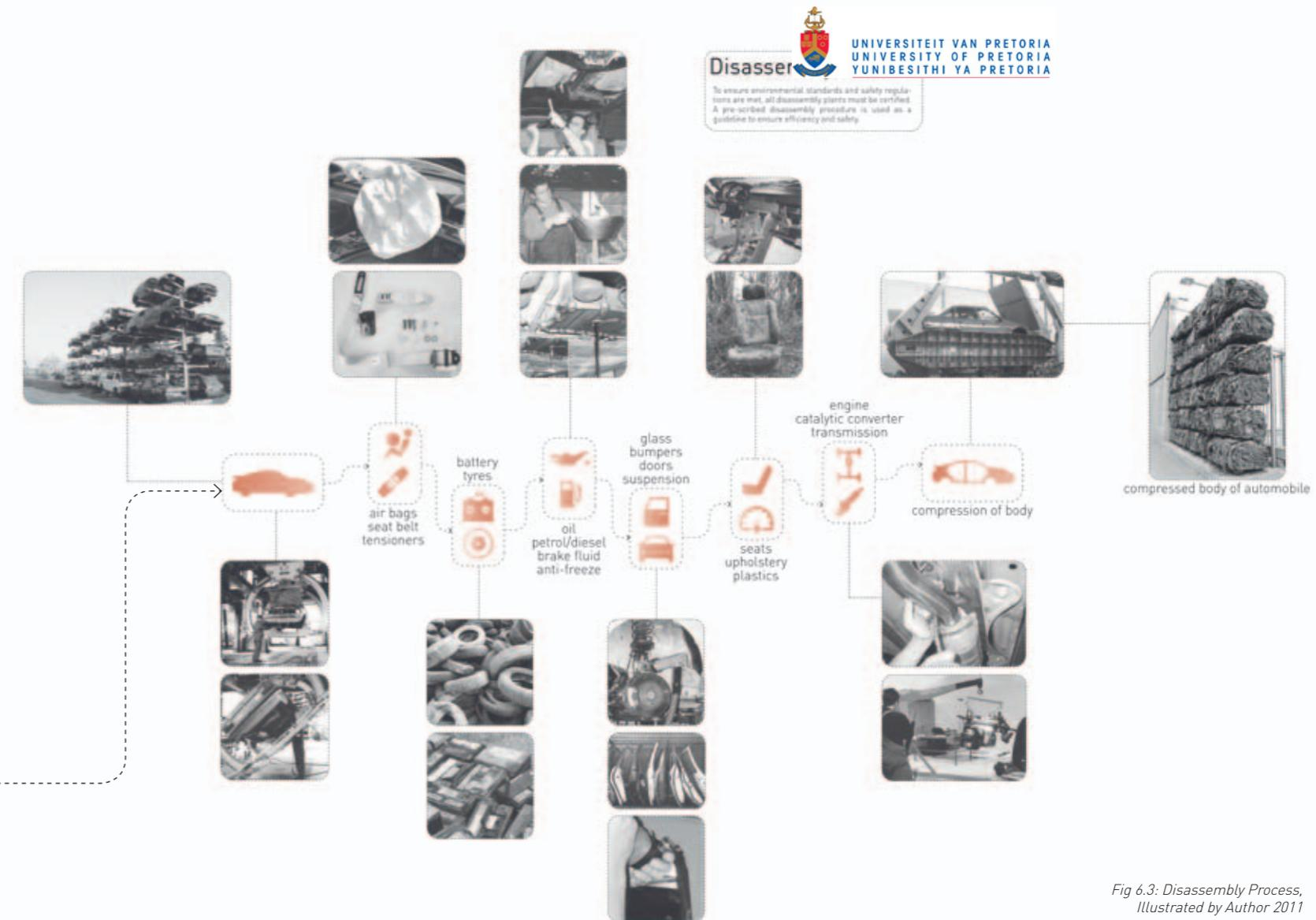
Fig 6.3: Disassembly Process, Illustrated by Author 2011
