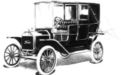
6-Passenger Town Car, Equipped with 3 Oil Lamps, Tubular Horn and Kit of Tools
