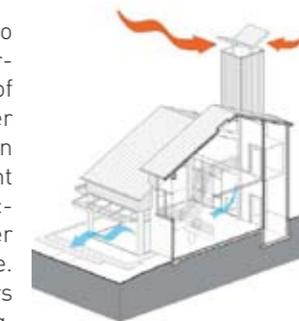
Fig 5.30: Cooling tower's ventilation diagram [Carboun 2010]
