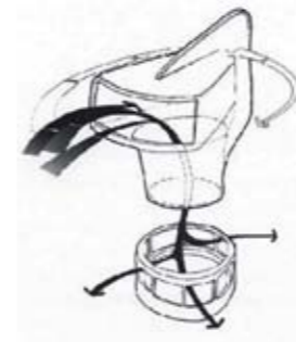
Fig 7.21: Wind scoop with pivot mechanism and fin (HVAC Systems 2001)
