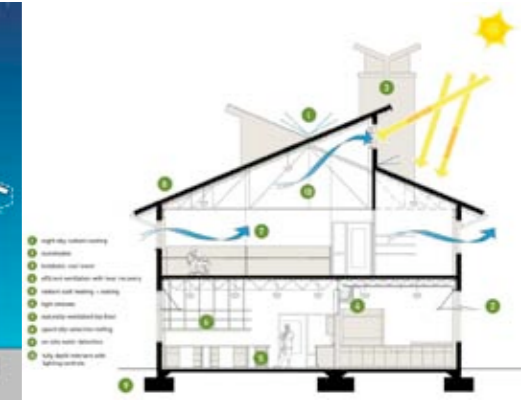
Fig 5.24: Section indicating sun angles and ventilation patterns (Carboun 2010)
