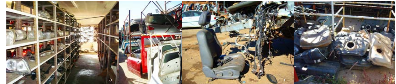
From left to right: a. Storage for smaller components b. Bonnet/boot storage racks c. Interior components and upholstery d. Petrol tanks
