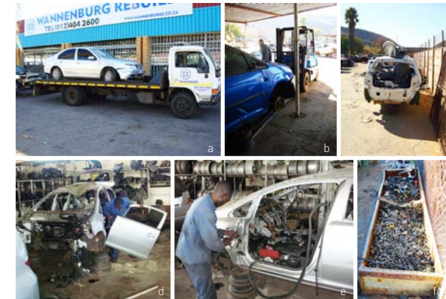
From top, left to right: a. Automobiles transported to site on flatbed trucks b. Forklift for moving automobiles in back yard c. Storage of disassembled vehicles before compression d/e. Disassembly of a vehicle f. Storage rack with different nuts and bolts
