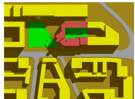
Figure. 134. 10 am sun on 21 June 2003 Four floors South wing
