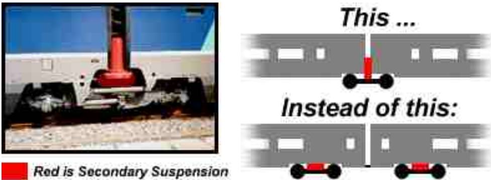
Figure 2.4. Explanation of the articulation of the trainsets in the TGV.
