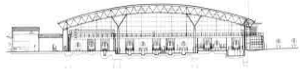
Figure 5.10.4. Above Section showing piling and column trees supporting space frame trusses. (World Architecture, April 1996:111)8
