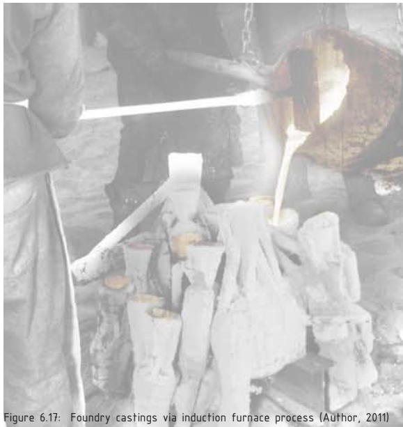
Figure 6.17: Foundry castings via induction furnace process (Author, 2011)
