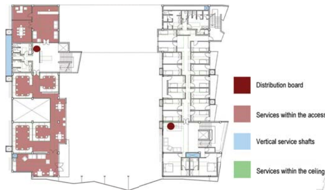
Fig. 7.37: Service distribution: fourth floor
