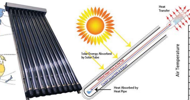
Fig. 7.16: Evacuated-tube solar collector
