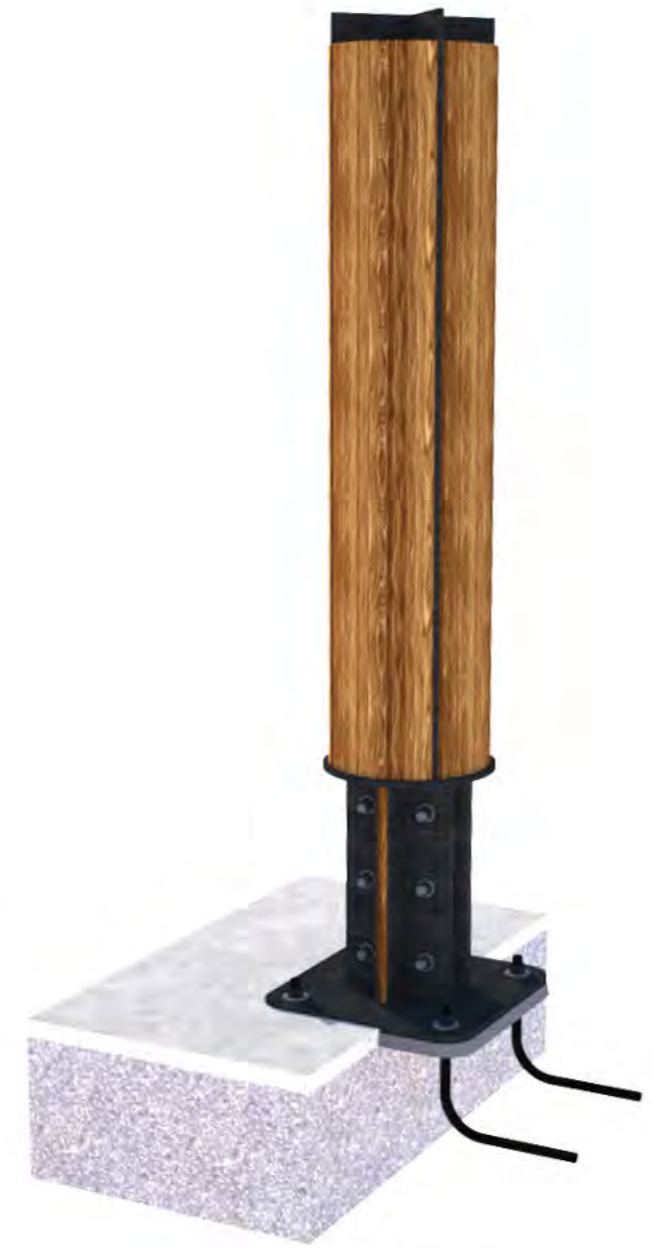
fig 166. Steel-timber composite footing detail. (not to scale)
