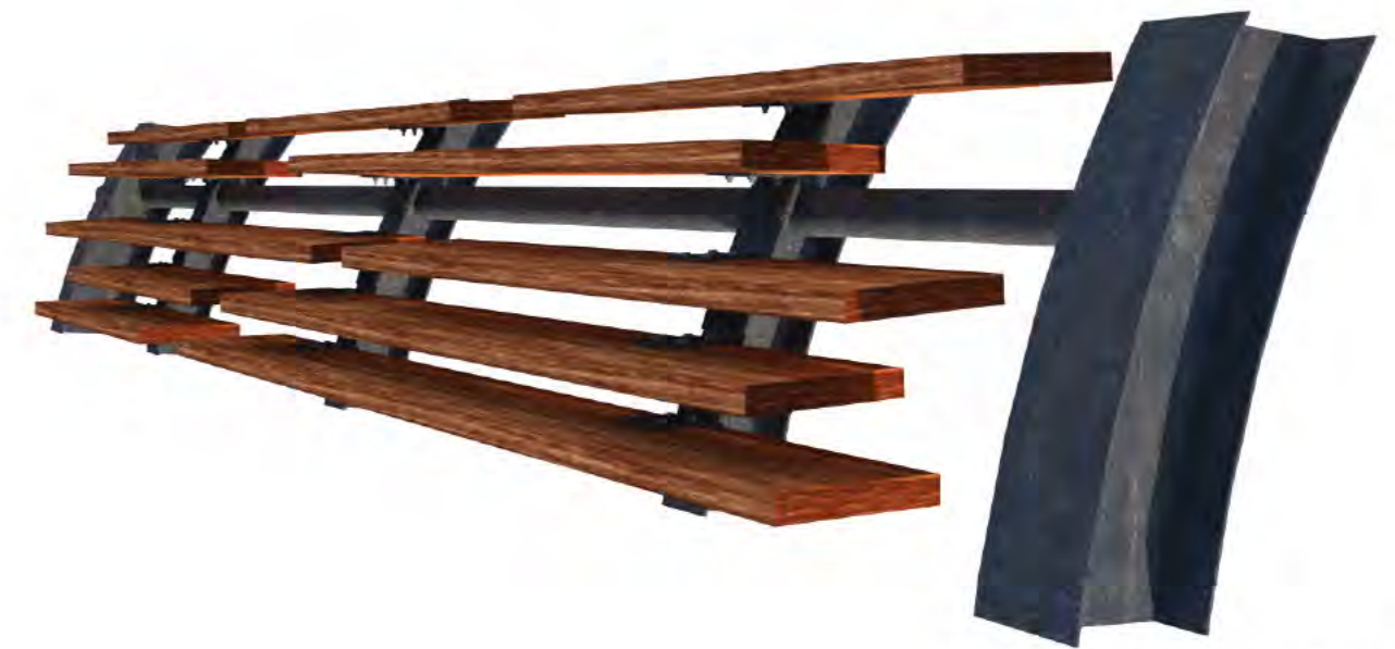
fig 174b. Detail of timber Scaffold screen.
