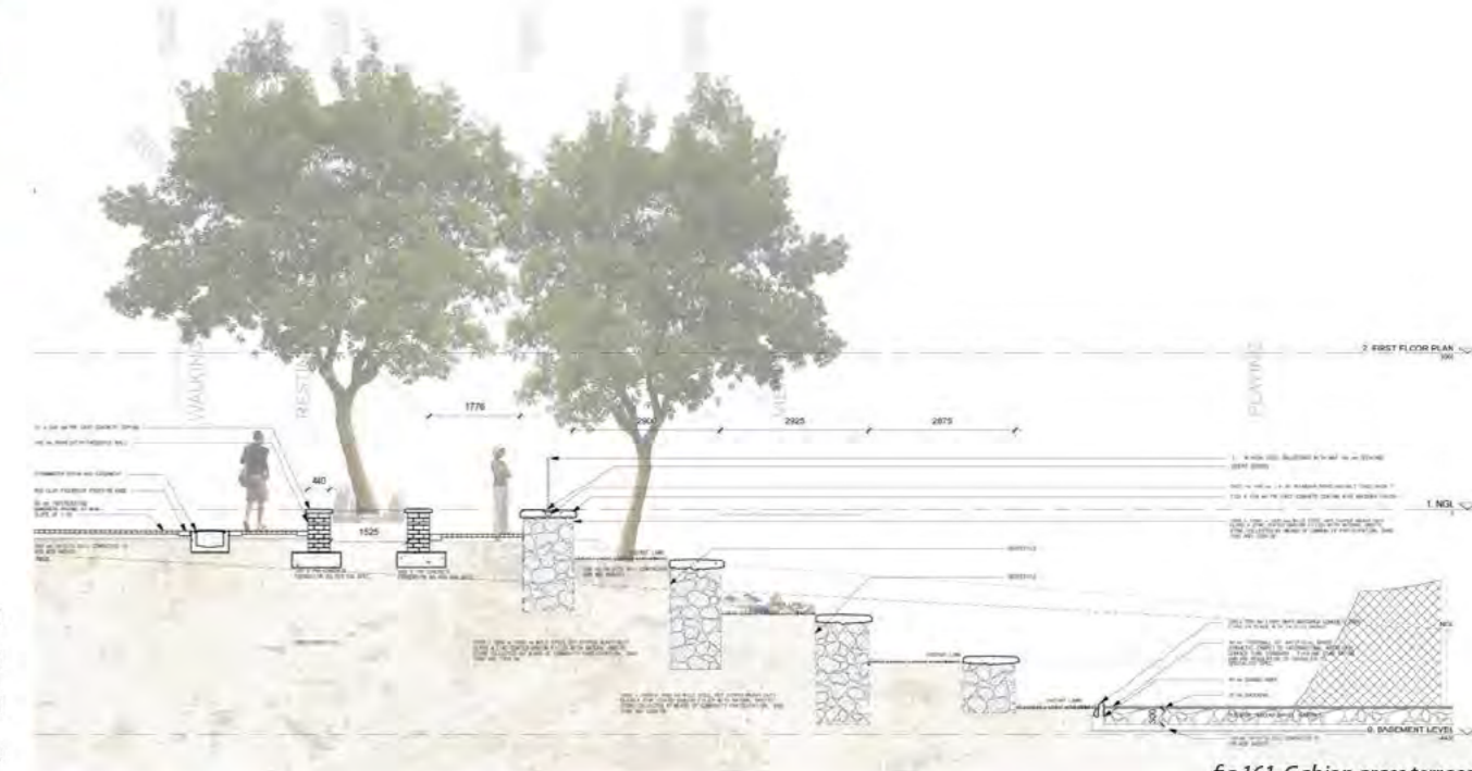
fig 161. Gabion grass terraces.
