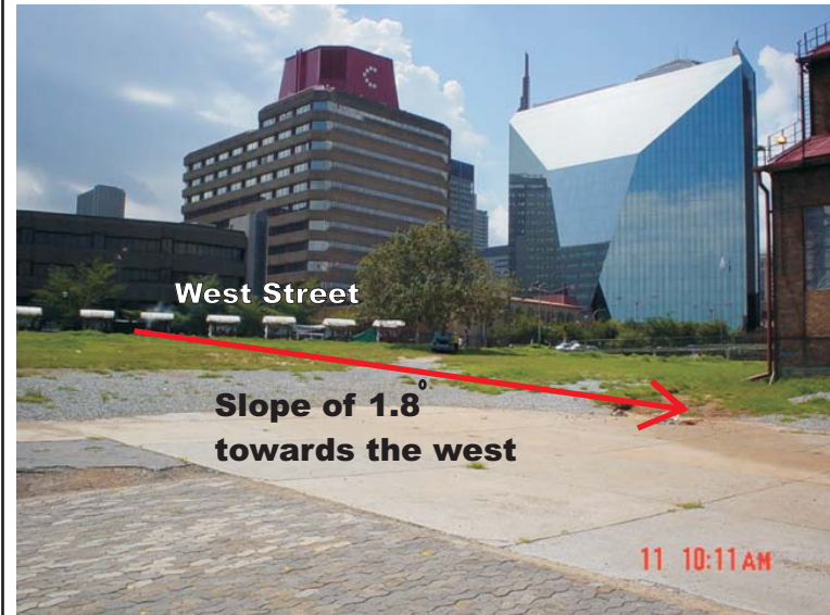
Fig 98. Site falls with slope of 1.8° towards the west.
